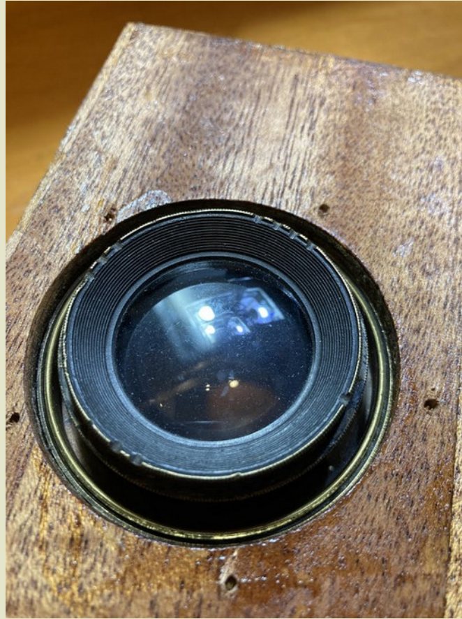
A Dallmeyer Lens with notches carved for “Soft Focus”
